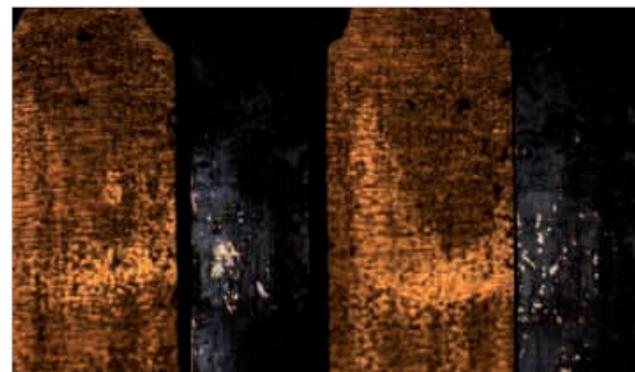
Test without GuideSpring: the gold pads show that the AdvancedMC™ has moved, ...
